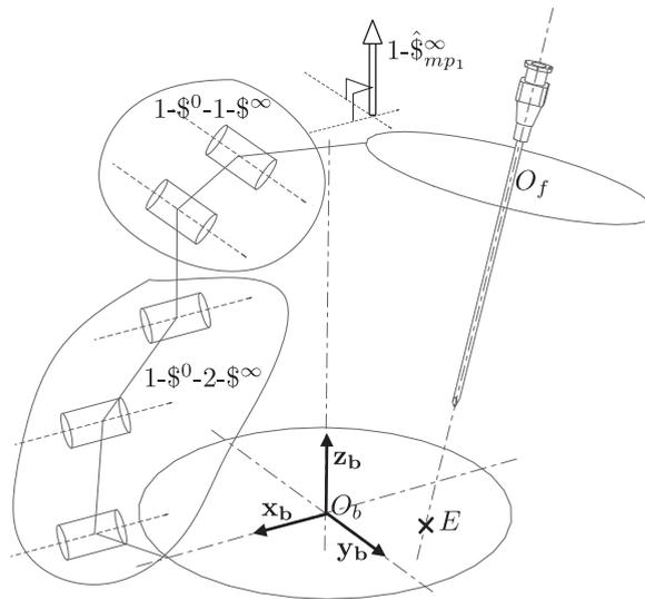
Fig. 7. Selected chain with wrench system  $1-1-1-3$ .
