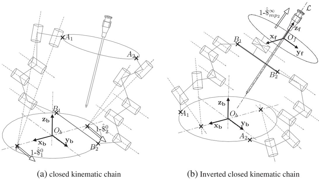
Fig. 10. Kinematic inversion.
